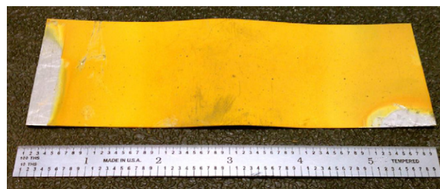
Fig. 2. The photographic image of as-sprayed \text{V}_2\text{O}_5 film (without binder and carbon) obtained by plasma spray deposition using solution precursor, \text{VOCl}_3 .
